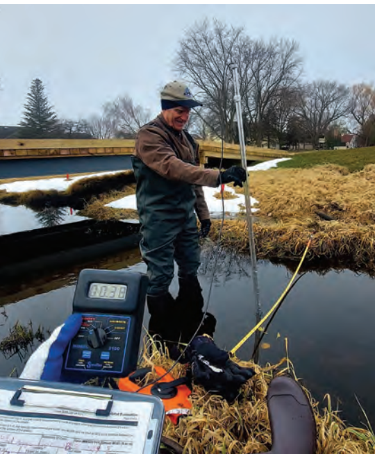
LLBMD Commissioner Jeff Bode volunteers to assist with gathering stream flow velocity data, which will be used to calculate total volume of water as well as Phosphorus load.
